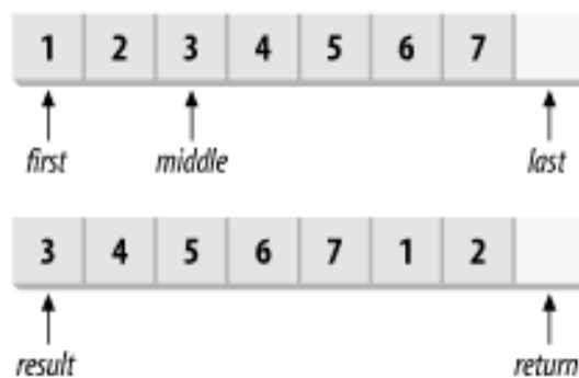
Figure 13-16. Rotating a range by two positions
